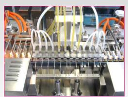
Filling through seal-less rotary piston pumps from ROTA: the volume to be filled is set through the colour touch-screen operator interface and can be stored in dedicated recipes.
