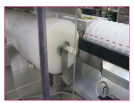
To allow a direct exit of the ampoules outside of the sterile room, the ROTA linear filling and sealing machines can be equipped on request with feeding screw systems at their outfeed, bringing the advantage to potentially avoid for example unnecessary sterilisation of collecting trays.
