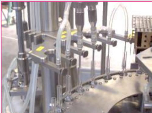
Ampoules are filled by mean of rotary piston pumps (accuracy better than  $\pm 0.5\%$ ). The ampoules are centered in order to allow the gassing and filling needles to move into the ampoules without touching their neck, so that wetted neck and black spots resulting from carbonisation are avoided. In order to increase the production flexibility, peristaltic pumps can optionnally be fitted to the machine.
