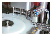
After the closing station, the filled and closed vials are gently pushed out of the transport star wheel by an exiting finger into the outfeed magazine, where they can be discharged by means of suitable trays.
