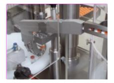
After the closing station, the filled and closed vias are gently pushed out of the transport star wheel by an exiting finger into the outfeed magazine, where they can be discharged by means of suitable trays.
