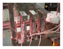
Vials are filled by mean of a rotary piston pump (accuracy better than  $\pm 0.5\%$ ). Depending on the vials to be processed and the requested output of the machine at large filling volume, the FLR50 can be equipped with up to four filling pumps respectively four filling stations. This ensures a large flexibility in terms of filling volumes, and high productivity from low to large volumes.
