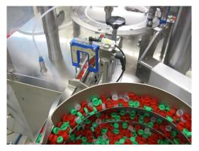
Micro-tubes are fed in bulk in the stainless steel sorting bowl, which transfers them over a vibrating rail to the main star wheel of the machine.
