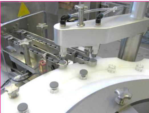
After the filling station, vial stoppering is performed through a pick & place arm, allowing full insertion as well as half insertion for vials to be freeze dried.
