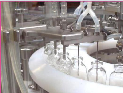
Vials are filled by mean of a rotary piston pump (accuracy better than  $\pm 0.5\%$ ). Depending on the vials to be processed and the requested output of the machine at large filling volume, the machine can be equipped with up to four filling pumps respectively four filling stations. This ensures a large flexibility in terms of filling volumes, and high productivity from low to large volumes.
