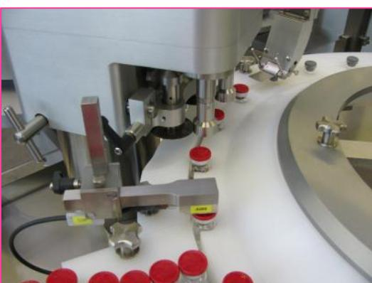
Once closed, the objects can be discharged from the outfeed magazine with suitable trays.
