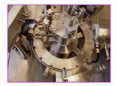
Ampoules are filled by mean of a rotary piston pumps (accuracy better than  $\pm$  0.5%).
