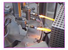
After the sealing station, the filled and sealed ampoules are gently pushed out of the transport star wheel by an exiting finger into the outfeed magazine.
