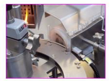
The inclined metal belt gently pushes the bunch of ampoules towards the infeed screw, which separates and transports them to the main star wheel. The transport star wheel hands gradually the ampoules over the machine through the opening station (option), filling station (pre-gassing, gassing during filling and post-gassing are optionally available) and sealing station. Thus a careful object transport is ensured.
