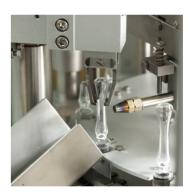
After the sealing station, the filled and sealed ampoules are gently pushed out of the transport star wheel into the outfeed magazine. The ampoules can then be discharged from the outfeed magazine by means of suitable trays or by hand.
