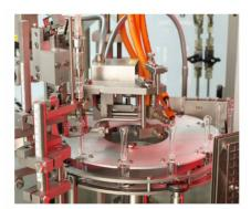
Ampoules are drop-free filled by mean of a seal-less rotary piston pumps (accuracy better than  $\pm$  0.5%).
