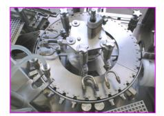
Ampoules are filled by mean of two rotarv piston pumps (accuracy better than  $\pm 0.5\%$ ). The ampoules are centred in order to allow the gassing and filling needles to move into the ampoules without touching their neck, so that wetted neck and black spots resultina from carbonisation are avoided.
