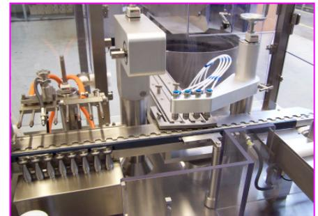
The inclined metal belt gently pushes the bunch of ampoules/vials towards the infeed screw, which separates and transports them to the intermediary wheel to be handed over to the transport rake. The transport rake hands gradually the ampoules/vials over the machine through the opening station (option), filling station (pre-gassing, gassing during filling and post-gassing are optionally available) and sealing station.
