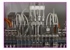
Ampoules are filled by means of four rotary piston pumps (accuracy better than  $\pm 0.5\%$ ). The ampoules are centred in order to allow the gassing and filling needles to move into the ampoules without touching their neck, so that wetted neck and black spots resulting from carbonisation are avoided.
