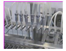
Ampoules are filled by means of six rotary piston pumps (accuracy better than  $\pm$  0.5%).
