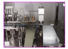
After the sealing station, the filled and sealed ampoules are gently pushed out of the transport rake by an exiting finger into the outfeed magazine.
