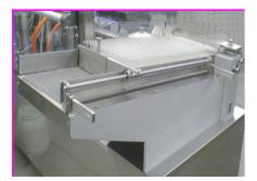
The inclined metal belt gently pushes the bunch of ampoules towards the infeed screw, which separates and transports them to the intermediary wheel to be handed over to the transport rake. transport rake The hands gradually the ampoules over the machine through the opening station (option), filling station (pre-gassing, gassing during filling and post-gassing are optionally available) and sealing station. Thus a careful object transport is ensured.
