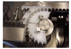
The inclined metal belt gently pushes the bunch of ampoules towards the infeed screw, which separates and transports them to the intermediary wheel to be handed over to the transport rake. transport rake hands The gradually the ampoules over the machine through the opening station (option), filling station (pre-gassing, gassing during filling and post-gassing are optionally available) and sealing station. Thus a careful object transport is ensured.
