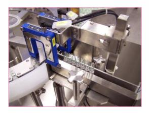
So-called "good" containers are driven into a stainless steel magazine, from which they can be collected in suitable trays. An optional rejection station collects all kind of rejected containers.
