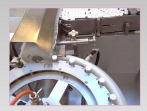
Containers are charged to the infeed magazine from trays. The magazine width is infinitely adjustable from 200 - 310 mm, the length is 445 mm.
