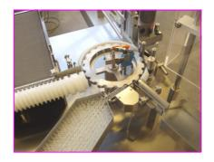
Containers are collected in an outfeed magazine of 153 mm outer width and 400 mm length. Different dimensions adapted to specific tray sizes are available. An optional rejection station collects all kind of rejected containers. When handling vials, the machine can be delivered with conveyor belt at infeed and/or outfeed in order to connect the machine with other processing machines like crimping machine upstream and blistering machine downstream.
