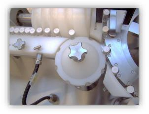
So-called "good" containers are positively driven by a vacuum star wheel and an outfeed screw into a stainless steel magazine, from which they can be collected in suitable trays.
