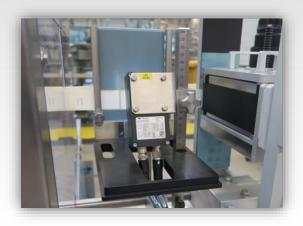
Starting from label presence sensor or pharma code reader to vision system for full print control, different type of sensors can be installed on the ROTA labelling machine to insure a full correctness of the labelling process.
