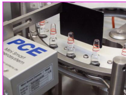
The machines are available with several sensors such as label presence, ampoule colour rings reader, vial cap colour reader, pharma code reader, print detection, etc...
