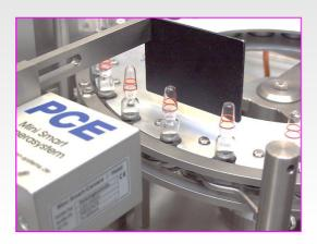
Starting from label presence sensor or pharma code reader to vision system for full print control, different type of sensors can be installed on the ROTA labelling machines to insure a full correctness of the labelling process.
