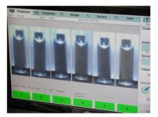
At the end of spinning, a light from the bottom illuminates the containers revealing the moving particles. The installed cameras are reproducing the real images of containers on the LCD screen, but magnified up to 9 times, depending on the container size. The operator can easily check them against particles and via suitable push buttons decide for their rejection.
