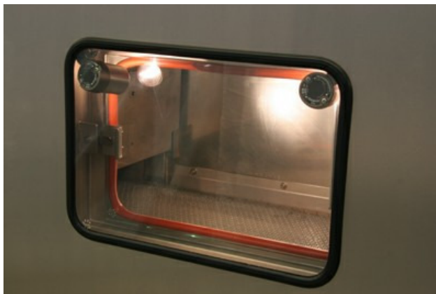
Inspection windows with lighting in infed and cooling zone
