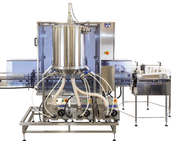
(Above) automation base with three Response units fitted, seen from the rear
