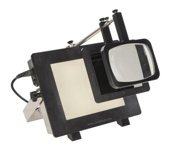
This polarised inspection light provides a simple method for the detection of visible particles in ampoules, vials and bottles. Particulate contamination of injections and intravenous infusions consists of extraneous, mobile, undissolved particles other than gas bubbles unintentionally present in the solutions.
