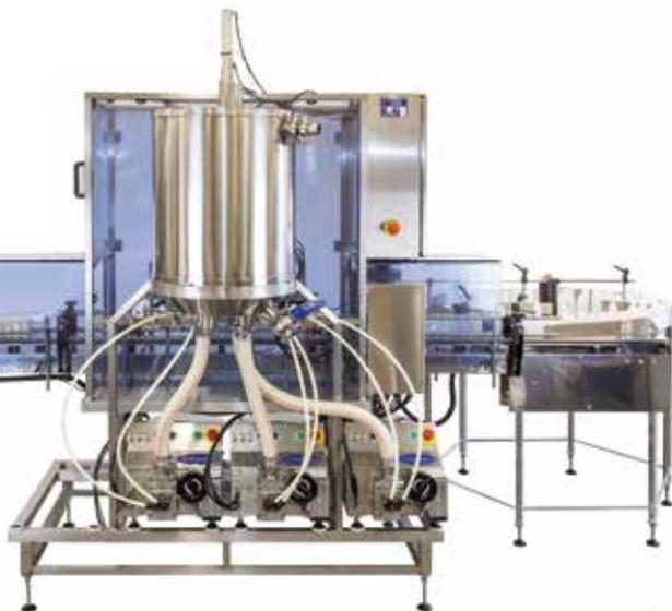
(Above) automation base with three Response units fitted, seen from the rear
