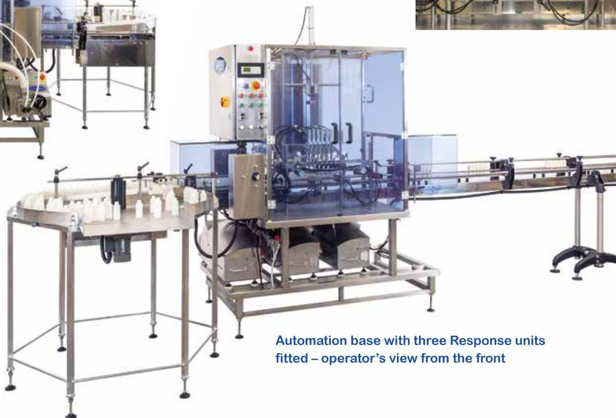
Automation base with three Response units fitted – operator’s view from the front
