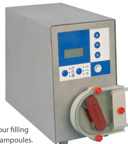
The Peristaltic Dispenser can be supplied with a range of sizes of high strength silicone tubing from 0.8mm bore to 8mm bore, with either a 1.6mm or 2mm wall thickness.
