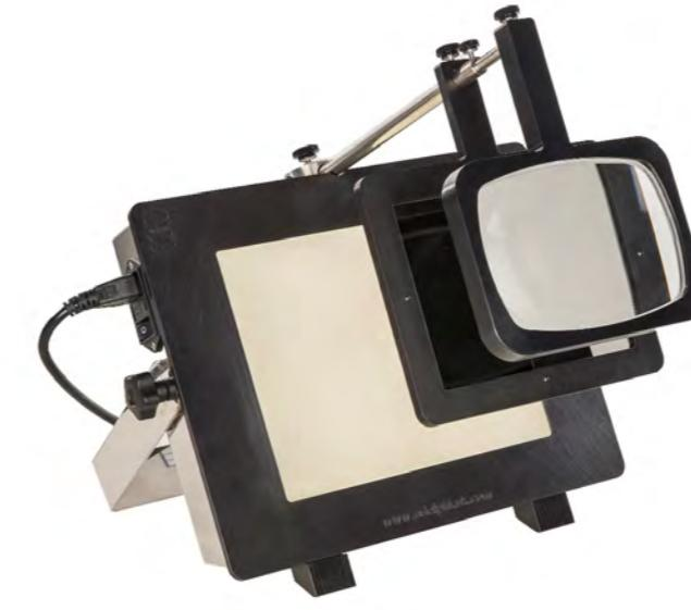
Designed for use in pharmaceutical and laboratory environments, the Apollo I Liquid Viewer has a polarised inspection light for the detection of particulate matter in transparent liquids contained in ampoules, vials and bottles. Particulate contamination can be unintentionally present in injections and intravenous infusions, and this unit provides a simple method of detection.
