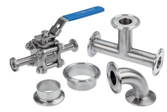
Our range includes 316L grade stainless steel fittings with outside pipe diameters from ½ inch to 4 inches. Gaskets are available in Silicone, Viton® and EPDM, and full material certification is available on all PHP Tri-Clamp fittings. All product contact surfaces have a surface roughness of 0.8Ra.
