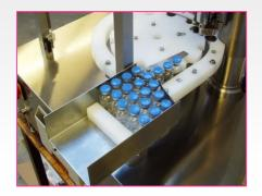
Vials are manually inserted by the operator into the transport star wheel, which hands gradually the vials over the machine through, for example considering machine type FLR25/G the filling station (pregassing, gassing during filling and post-gassing are optionally available), and the rubber stoppering station.
