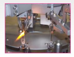
Ampoules are manually inserted by the operator into the transport star wheel, which hands gradually the ampoules over the machine through the opening station (option), filling station (pregassing, gassing during filling and post-gassing are optionally available) and sealing station. Thus a careful object transport is ensured.
