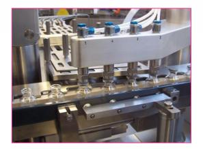
The infeed metal belt gently pushes the bunch of ampoules towards the infeed screw, which separates and transports them to the intermediary wheel to be handed over to the transport rake.
