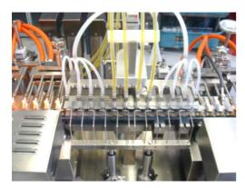
Filling through seal-less rotary piston pumps from ROTA: the volume to be filled is set through the colour touch-screen operator interface and can be stored in dedicated recipes.
