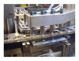
In addition to ampoule filling and sealing, the machine is equipped with a rubber stopper sorting and feeding station for vials. Stoppers are inserted (full or half-insertion) using a pick & place arm.
