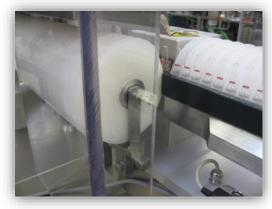
The infeed metal belt gently pushes the bunch of ampoules towards the infeed screw, which separates and transports them to the intermediary wheel to be handed over to the transport rake.
