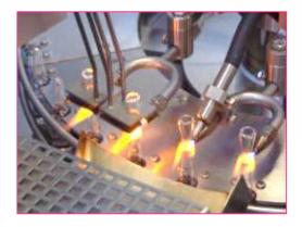
After the flame sealing station, the filled and sealed ampoules are gently pushed out of the transport star wheel by an exiting finger into the outfeed magazine.
