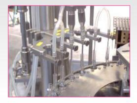
Ampoules are filled by mean of rotary piston pumps (accuracy better than  $\pm$  0.5%).
