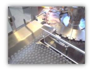
The inclined metal belt gently pushes the bunch of ampoules towards the infeed screw, which separates and transports them to the main star wheel. The transport star wheel hands gradually the ampoules over the machine through the opening station (option), filling station (pre-gassing, gassing during filling and post-gassing are optionally available) and sealing station. Thus a careful object transport is ensured.
