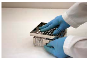
1. Unscrew 2 thumbscrews holding Orientor Tray to Base.
