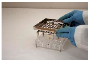
2. Position new Orientor Tray and secure with 2 thumbscrews.
