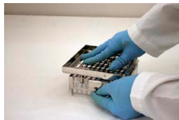
1. Unscrew 2 thumbscrews holding Orienter Tray to Base.
