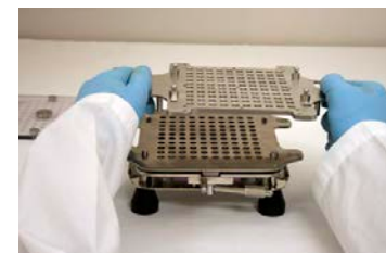
7. Place new size Caps Tray onto Filler. You are now ready to fill a new capsule size.
