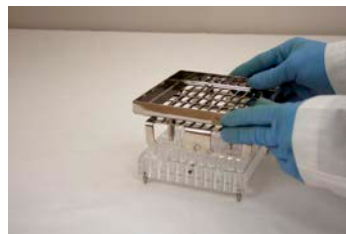
2. Position new Orienter Tray and secure with 2 thumbscrews.
