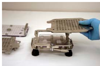
4. Set Cam Lever to 3 o'clock. Remove the 3 Body Sheets.
