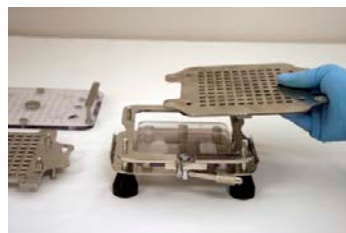
6. Place new size Body Sheet "a" then "b", then "c" on locating pins.
