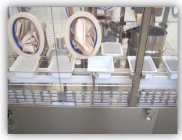
The ROTA syringe machines feature the use of the latest servo motor technology and machine components of the latest generation. Serial kinematics robotics (SCARA) and advanced control programming allow the precise execution of each individual processing steps, avoiding syringe damages and allowing precise and problem free filling and rubber stoppering.
