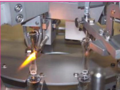
Ampoules are manually inserted by the operator into the transport star wheel, which hands gradually the ampoules over the machine through the opening station (option), filling station (pre-gassing, gassing during filling and post-gassing are optionally available) and sealing station. Thus a careful object transport is ensured.
