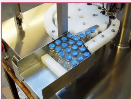
Vials are manually inserted by the operator into the transport star wheel, which hands gradually the vials over the machine through, for example considering machine type FLR25/G the filling station (pre-gassing, gassing during filling and post-gassing are optionally available), and the rubber stoppering station.
