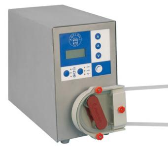
The Accuramatic Peristaltic Dispenser can be supplied with a range of sizes of high strength silicone tubing from 0.8mm bore to 8mm bore, with either a 1.6mm or 2mm wall thickness.
