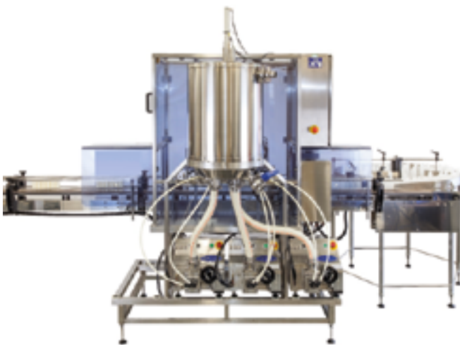
(Above) Automation Base with three Response units fitted; seen from the rear
