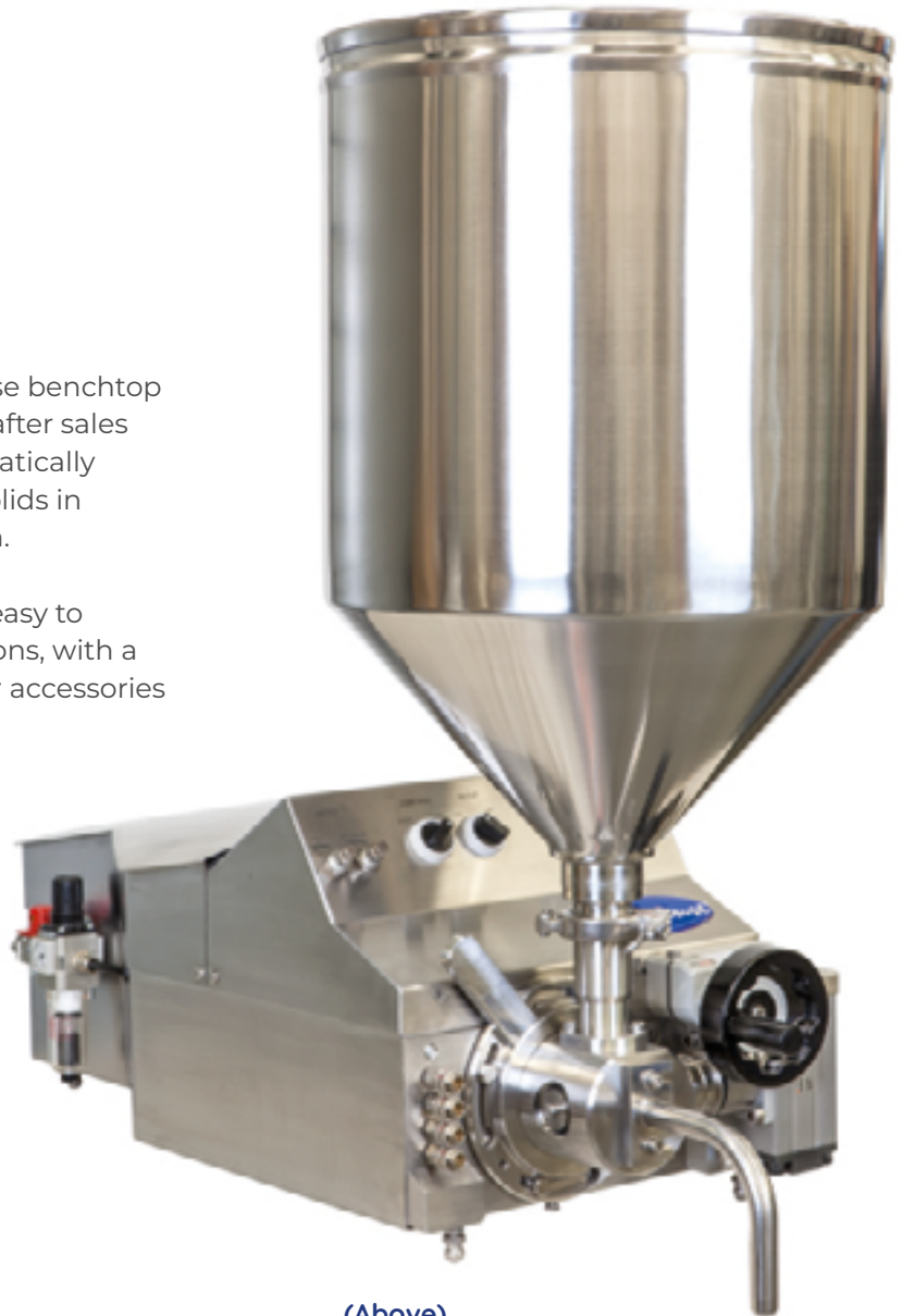
(Above) With standard hopper for filling creams, pastes, and solids in suspension
