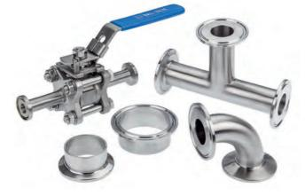
Our range includes 316L grade stainless steel fittings with outside pipe diameters from ½ inch to 4 inches. Gaskets are available in Silicone, Viton® and EPDM, and full material certification is available on all PHP Tri-Clamp fittings. All product contact surfaces have a surface roughness of 0.8Ra.
