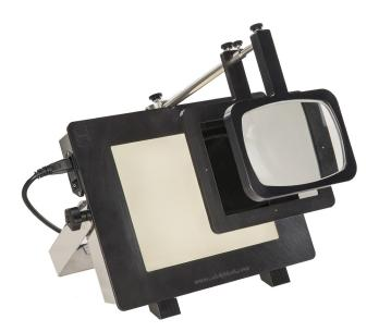
Designed for use in pharmaceutical and laboratory environments, the Apollo I Liquid Viewer has a polarised inspection light for the detection of particulate matter in transparent liquids contained in ampoules, vials and bottles. Particulate contamination can be unintentionally present in injections and intravenous infusions, and this unit provides a simple method of detection.
