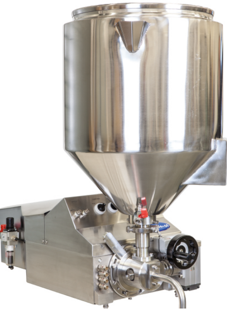
Left: heated hopper for hot fills.
